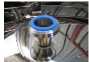
DN38 SMS wash ball connection on 40 cm diameter cover
